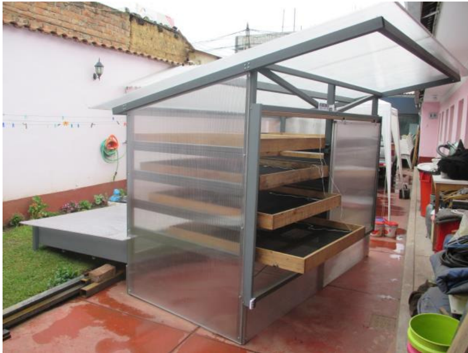
Prototype of solar cacao dryer.
