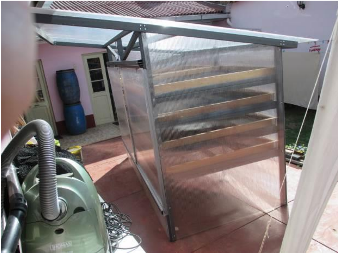
Tower section of the solar cacao dryer.
