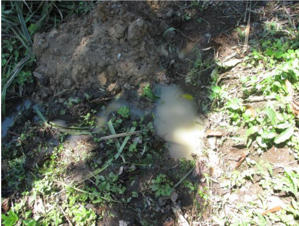
Water flowing from test hole 24 hours after excavation.
