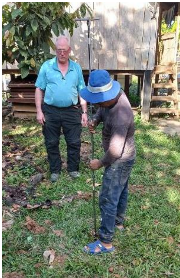
Arthur and Jorge drilling test boring.
